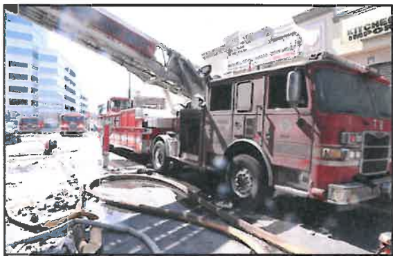
Aerial Ladder Truck Tractor and Trailer damage
