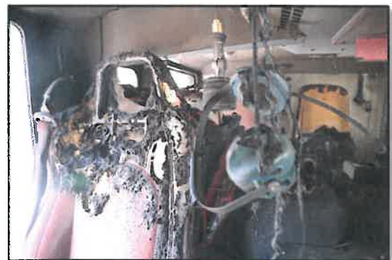
Aerial Ladder Truck Interior Cab damage
