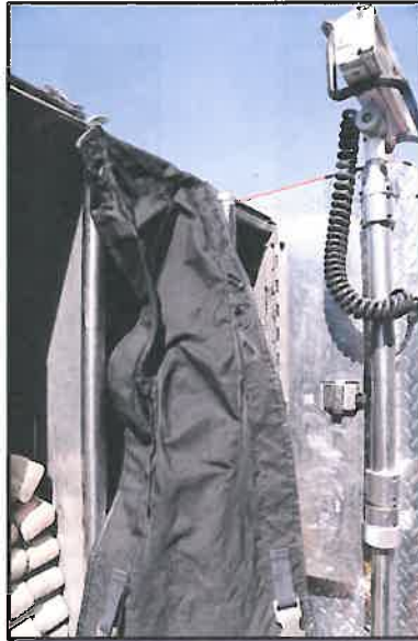
Engine hose cover damage
