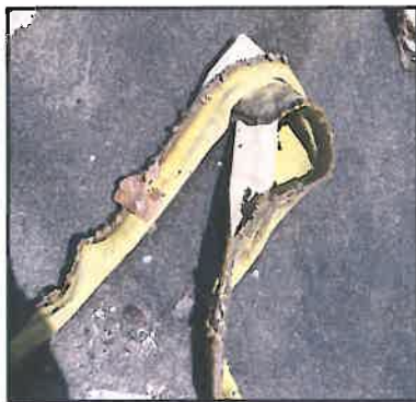
1 3/4" hose line damage
