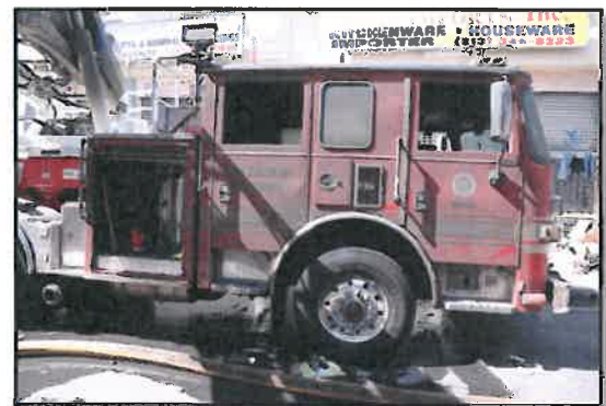
Aerial Ladder Truck Exterior Cab damage
