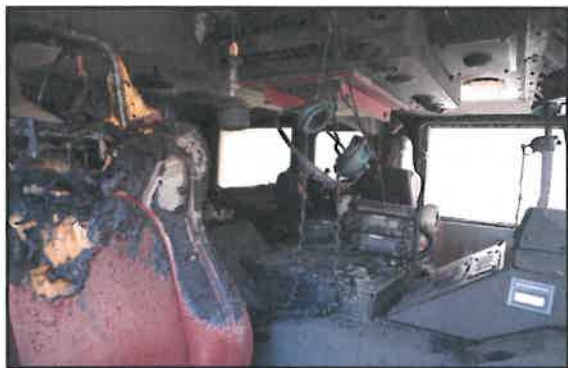
Aerial Ladder Truck Interior Cab damage
